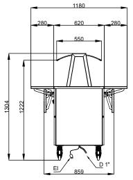
Drain Electrical inlet (power)
